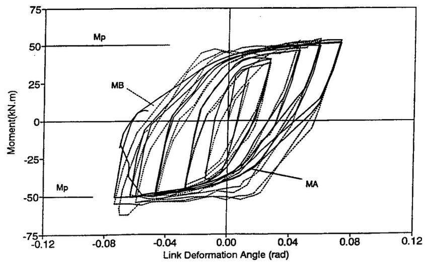
Fig. 2 Moment-link deformation angle hysteresis loops for specimen 3
