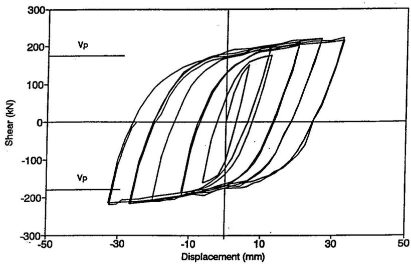
Fig. 4 Shear-displacement hysteresis loops for specimen 5
