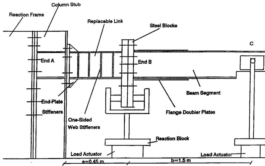
Fig. 1 Schematic of test setup
