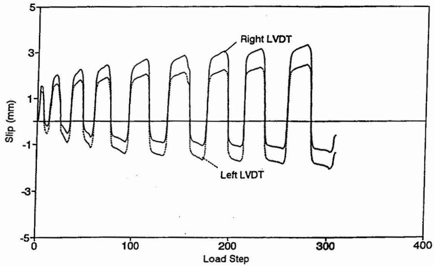
Fig. 6 Variation of vertical slippage with loading steps for specimen 3
