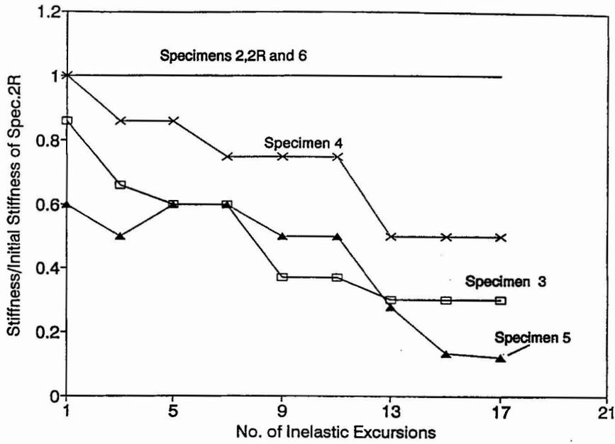
Fig. 5 Variation of connection stiffness  $K$  as a percentage of initial stiffness  $K_{2R}$  of specimen 2R
